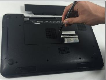
• Remove the 5 mm Phillips # 0 screw in the middle of the device.
