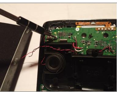
Remove the five 6mm T6 screws connecting the circuit board to the rear panel.
