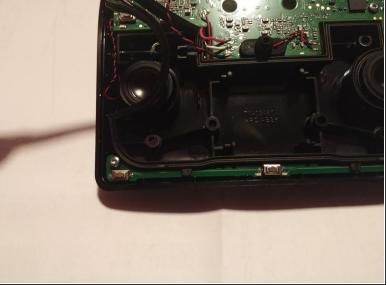
Remove the rubber gasket using tweezers.
