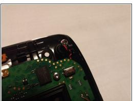
Remove the microphone from microphone slot.
