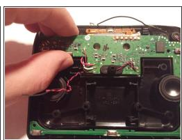
Carefully use the plastic opening tool to lift the circuit board up.
