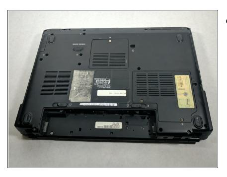
Remove the battery from the slot.
