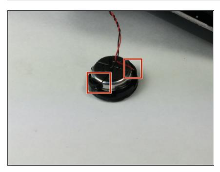
Desolder the two wires connecting to the speaker.
