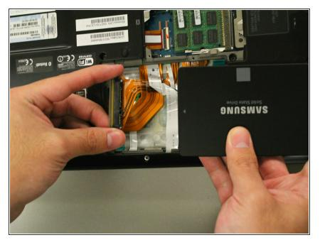
Connect the drive (in this case a solid state drive) to the laptop using the SATA cable located inside the hard drive placement area.
