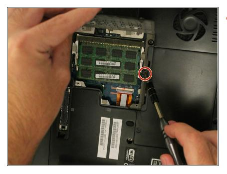
Lift and remove the RAM cover to reveal the first of 2 40mm screws holding down the hard drive cover. Remove the screw using a Phillips #00 Screwdriver.
