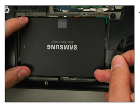
Once the drive is connected, carefully insert the drive into the laptop enclosure.
