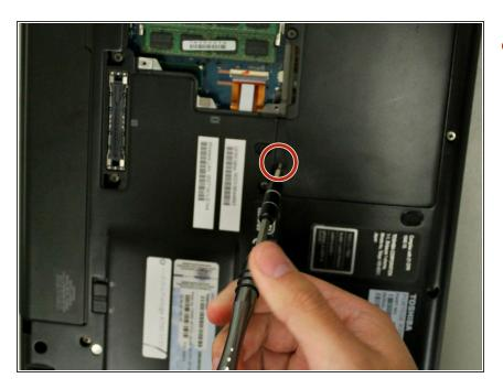
Remove the second 40mm hard drive cover screw using a Phillips #00 Screwdriver.
