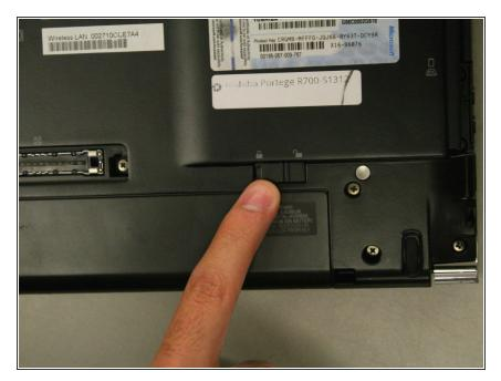
• Locate the battery lock button and push it towards the unlock position.
