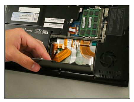
• Lift and remove the hard drive cover.
