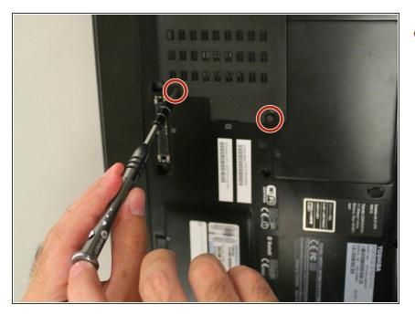
Remove the 40 mm screws from the RAM cover using a Phillips #00 Screwdriver.
