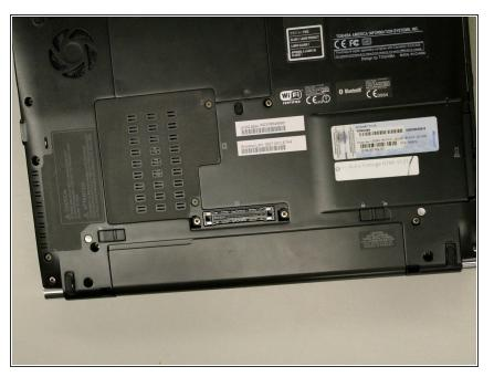
• Locate the battery on the backside of the laptop. The battery is usually located at the bottom.
