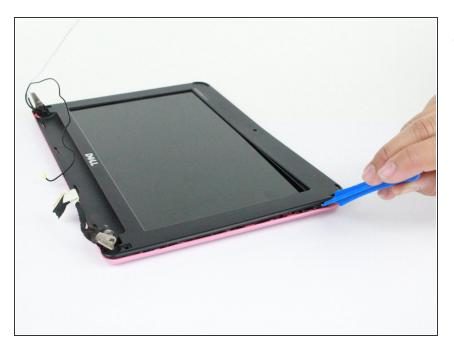
Using the plastic opening tool gently pry up the inside edge of the display bezel.
