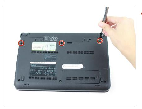
Remove the three 8mm Philips 0 screws securing the keyboard.
