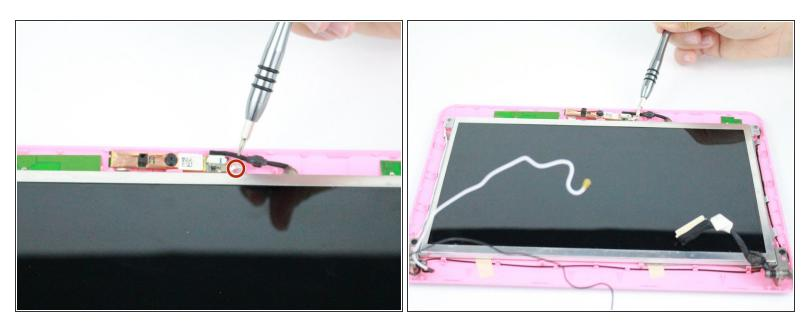
• Remove the single 3mm Phillips screw securing the camera to the display panel.
