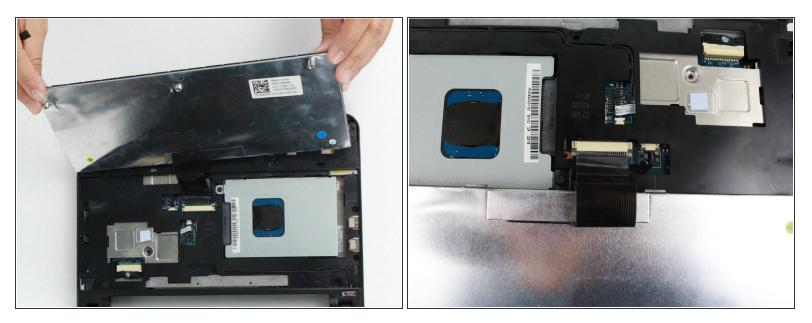
Lift the keyboard off of the support bracket carefully since it is still connected by a ribbon cable.
