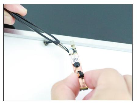
Disconnect the camera cable using tweezers.
