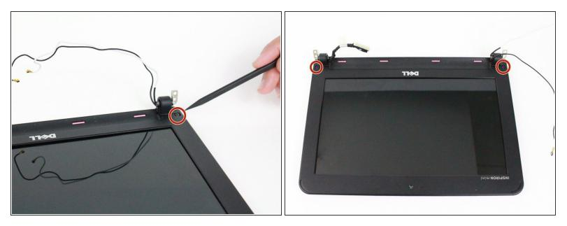
• Remove the two 4 mm Phillips 0 screws on the display bezel.
