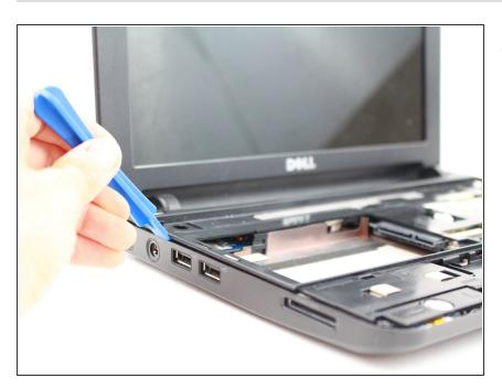
Gently pry off the bracket using the prying tool.
