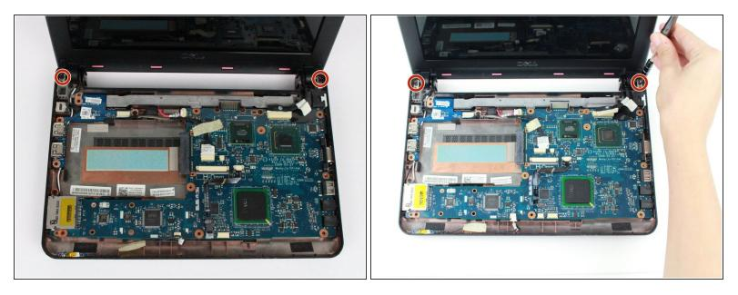
• Remove the two 4 mm Phillips 0 screws that secure the display assembly to the computer base.
