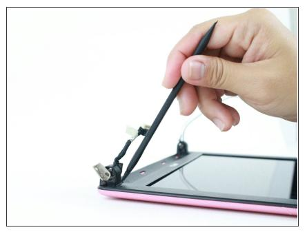
• Press and remove the hinge cover caps using the spudger.
