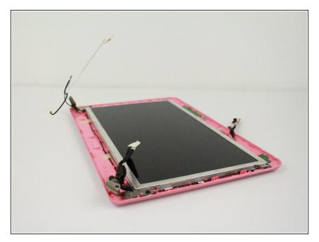
Remove the display bezel using a plastic prying tool.
