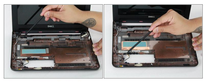
Pull the Mini-Card cables out of the computer base. They slide out from under a few pieces of plastic that secure them to the base.
