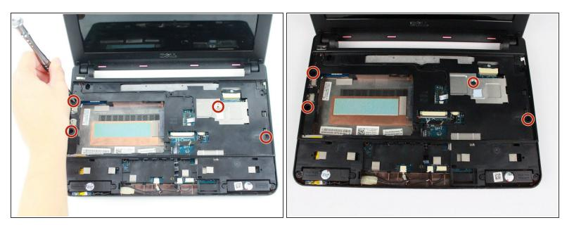
Remove the four 6mm Philips 0 screws securing the bracket.
