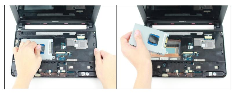
• Pull on the black tab and slide the hard-drive cage toward the USB port on the left side of the device until its comes free and carefully lift out of device.
