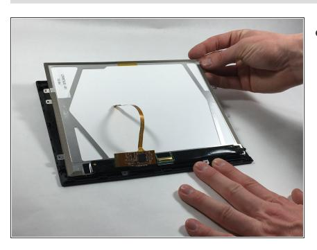
Lift and carefully remove the LCD display from the front cover.
