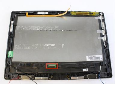
Open the latch on the copper connector and remove it from the tablet.
