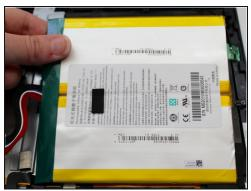
• Use the plastic opening tool to separate the glue that holds the battery to the screen.
