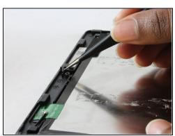
• Remove the three small latches that are underneath the screws.
