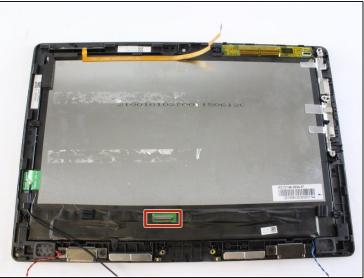
• Open the latch on the copper connector and remove it from the tablet.
