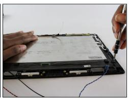
• Remove the three 3.5mm screws from the outside perimeter of the tablet.
