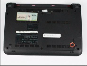
On the bottom of the laptop locate the removable panel and screw holding it to the body. Loosen the screw and take the cover off.
