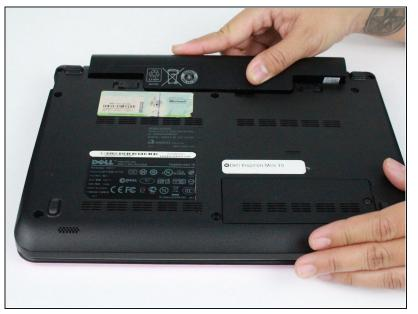
• Remove the battery by pulling it up and out.
