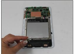
• Lift the white bar on the ZIF connector and pull the metal connector out.
