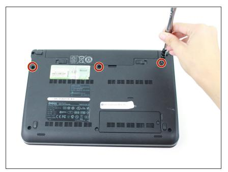
Remove the three 8mm Philips 0 screws securing the keyboard.
