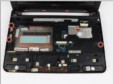
Remove the four 6mm Philips 0 screws securing the bracket.
