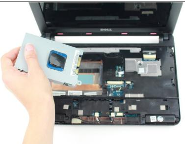
Pull on the black tab and slide the hard-drive cage toward the USB port on the left side of the device until its comes free and carefully lift out of device.
