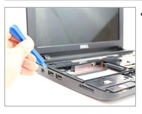
Gently pry off the bracket using the prying tool.
