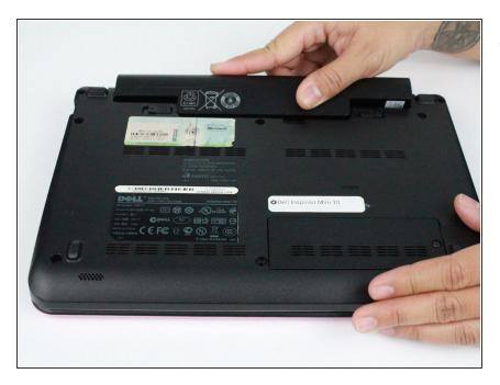
Remove the battery by pulling it up and out.
