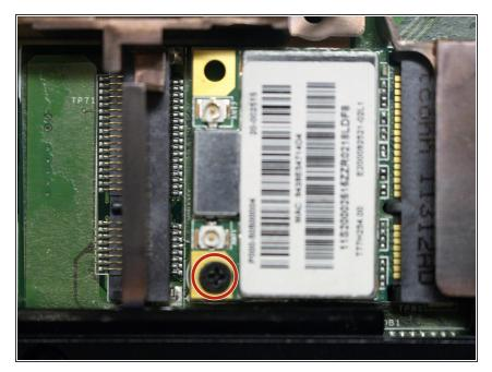
Using the Phillips #00 Screwdriver, remove the one 3.4 mm screw from the Wi-Fi card.
