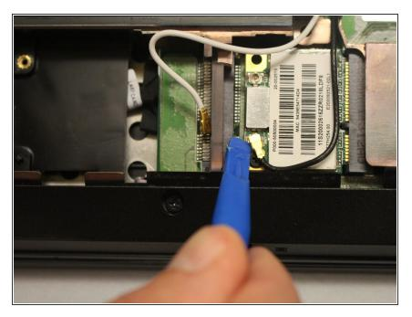
Using the plastic opening tool, detach both black and grey cables from the Wi-Fi card.
