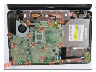
Use the Phillips PH00 to unscrew the fifteen 4mm screws holding down the motherboard.
