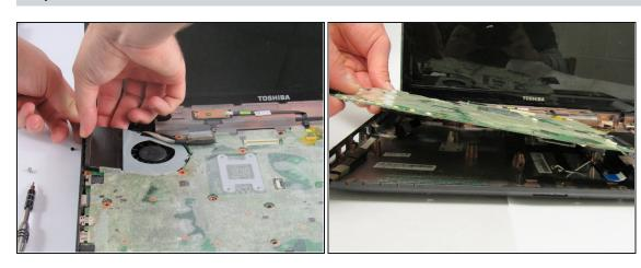
• Lift the motherboard and disconnect the 4 pin connector on the bottom side.
