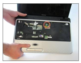
Remaining is the cord that connects the keyboard to the motherboard.
