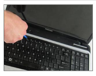
Using the plastic opening tool carefully pry the plastic strip that sits at the top of the keyboard.
