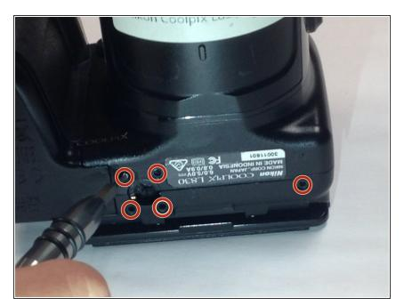
Unscrew the five 3.0mm Phillips #000 screws that are located on the bottom side of the camera.
