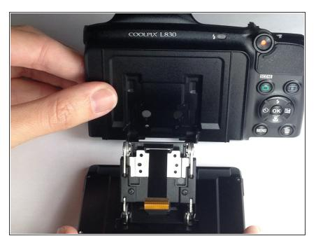
Gently pull the ribbon connector in order to remove the complete LCD Monitor Connecting Arm.
