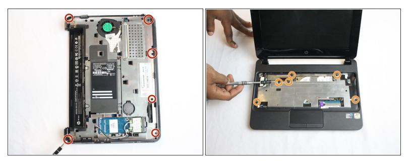
• Remove the six black screws around the perimeter of the laptop using a Phillips #1 screwdriver.
