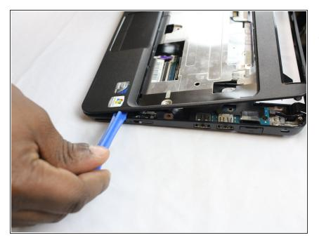
Lift the keyboard bezel from the back end and slide the iFixit opening tool around the perimeter of the bezel until it is fully released.
