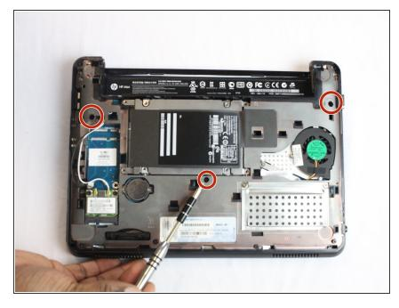
Remove the three black screws marked by the keyboard symbol using a Phillips #1 screwdriver.
