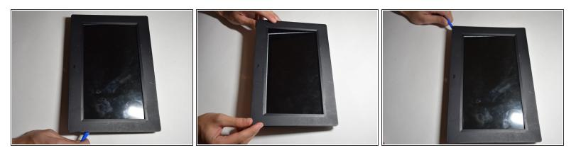
• Using the black nylon spudger, pry off the clips all around the frame. You will hear a popping sound for every clip
