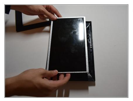
• Lift screen out of place so you can access the plugs that connect it.
