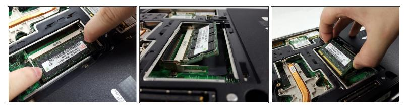
• If necessary, repeat this process with the second RAM stick that lies beneath the first one.
