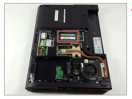
The RAM sticks are located near the center of the device, and are arranged one on top of the other.
