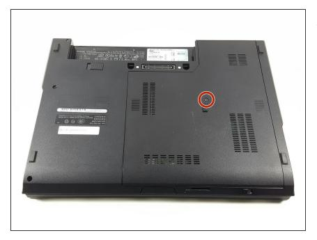
Unscrew the single 3.5mm Phillips #1 screw that holds on the bottom plate of the device.
