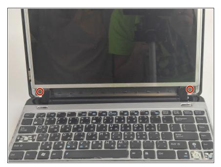
After removing the cover, remove the two 4.6mm screws using the J0 Phillips head screwdriver.
