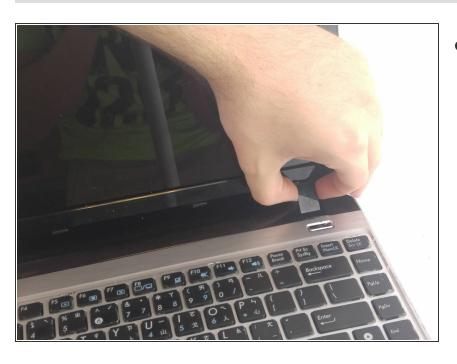
You must separate the hinge cover from the cover before removing the cover.
