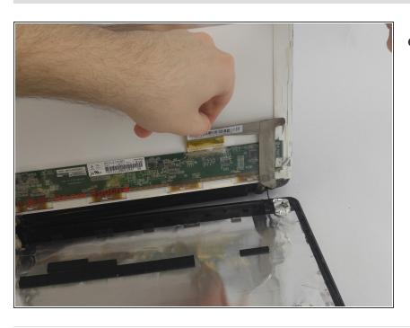
Pull up on the video cable on the back of the LCD display to remove it.
