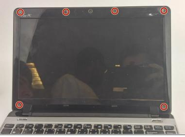
Remove the six screw on the front cover by using the plastic opening tool. Then, remove the six
