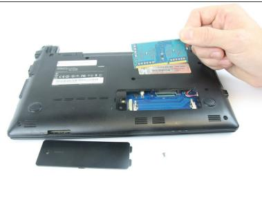
Finally, use the black spudger to get underneath the loosened RAM chip and gently pull it up and out of the laptop. To reassemble your device, follow these instructions in reverse order.
