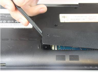
• Insert the flat end of the black spudger into the small notch in the RAM slot and lift the top off.
