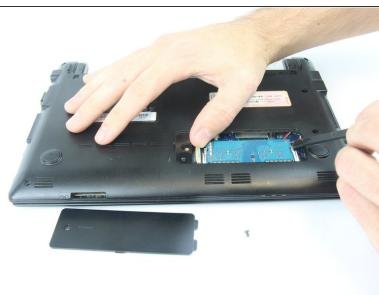
Now that the RAM chip has been exposed, use your fingertip and the black spudger to push back the metal tabs on each side, allowing the RAM chip to come free.
