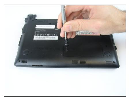
Use a Phillips #0 screwdriver, take out the 4.6mm screw holding the RAM slot down.
