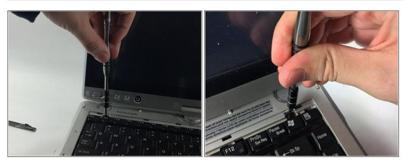
Remove the two screws with a phillips head screwdriver. Be careful not to lose the screws.
