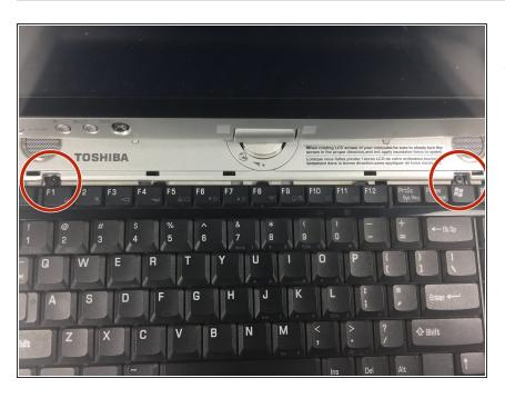
Locate the two screws on each side.
