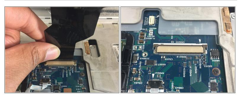
Disconnect the keyboard from the laptop by unplugging the power ribbon.
