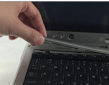
First, begin by removing the plastic cover that is located at the top of the keyboard. This can be pried off or just removed by hand by grabbing the plastic piece by the indent on either side and lifting up.
