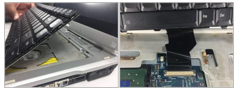
Lift the keyboard up to reveal the power plug.
