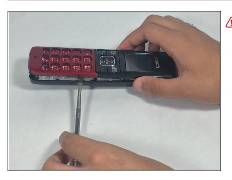
After removing the two screws from the back of the phone carefully use the metal spudger to lift along the edges and raise the phone case from the internal clips.
