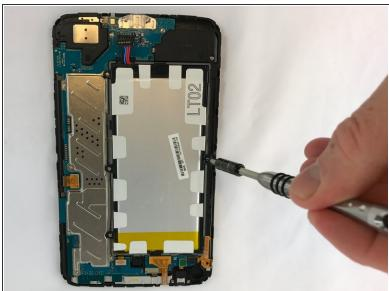
Remove the four 1.2 mm Phillips #000 screws surrounding the battery.
