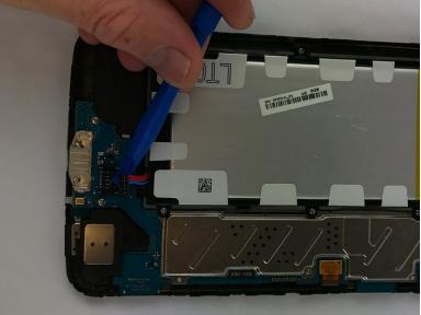
Unplug the battery connection carefully using the plastic opening tool.
