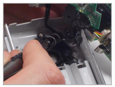
• Unscrew the camera housing unit from the plastic case.
