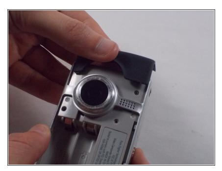
• Slide the black upper casing off from the device.
