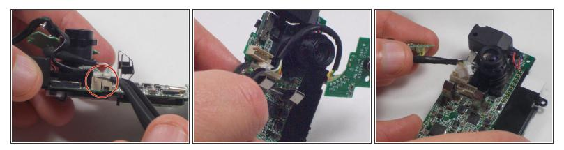
• With tweezers, remove the microphone and USB connections.
