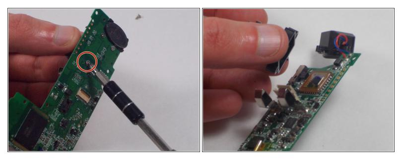
Remove the single 2.1 mm screw and separate camera from the circuit board.
