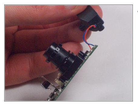
• Camera lens is now separated from the circuit board.
