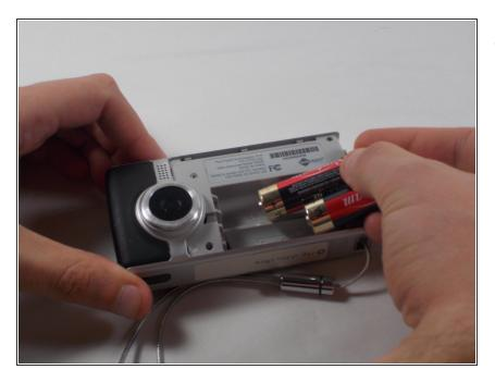
• Remove the batteries
