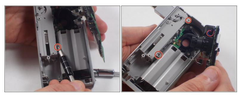
• Unscrew the single 1mm screw from USB housing unit.
