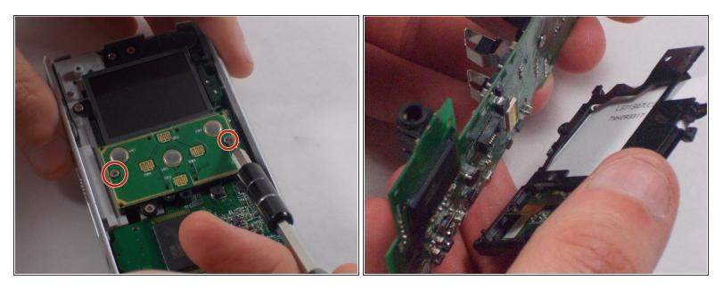
• Unscrew the two 1mm screws from the board shown. Remove screen from circuit board.
