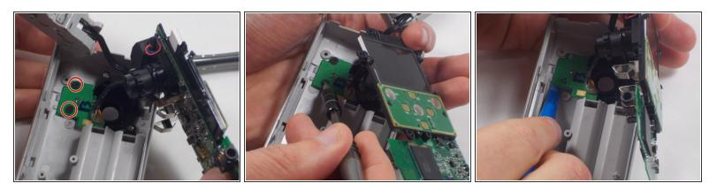
• Remove the two 1mm screws and separate the circuit board and camera from the plastic casing.
