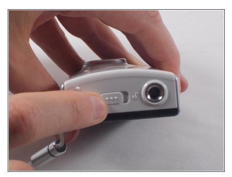
Unlock the battery cover by sliding the switch to the unlock position.
