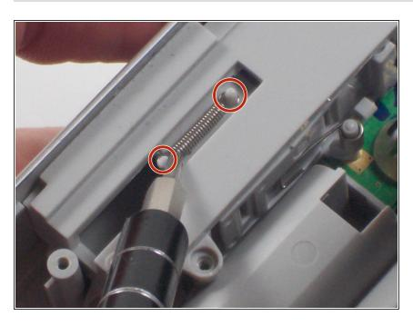
Using the Phillips head screwdriver, disconnect spring from the plastic nubs.
