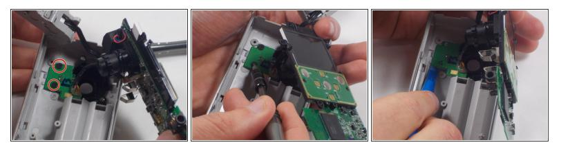
• Remove the two 1mm screws and separate the circuit board and camera from the plastic casing.
