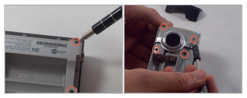
• Remove the six 1mm screws from the back and upper casing with the Phillips Head screwdriver.
