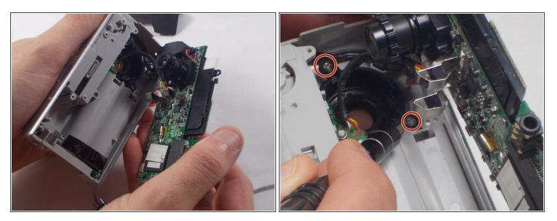
Unscrew the 2 1mm screws and gently separate camera wires from plastic casing.
