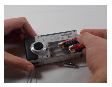
• Remove the batteries
