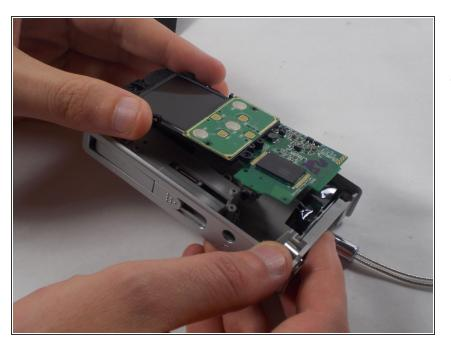
• Gently separate the circuit board from the casing.
