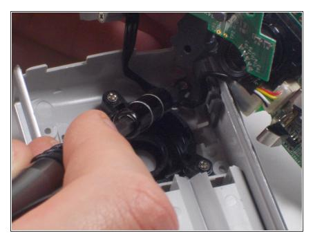
• Unscrew the camera housing unit from the plastic case.
