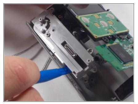
• Gently pry out the USB housing unit with the Ifxit Opening Tool.
