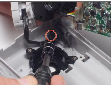
Remove the three 1mm screws from the USB connector and back casing with the Phillips Head screwdriver.
