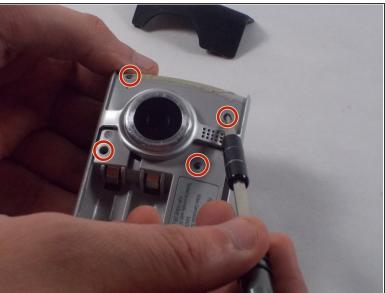
Remove the six 1mm screws from front of the camera with the Phillips Head screwdriver.
