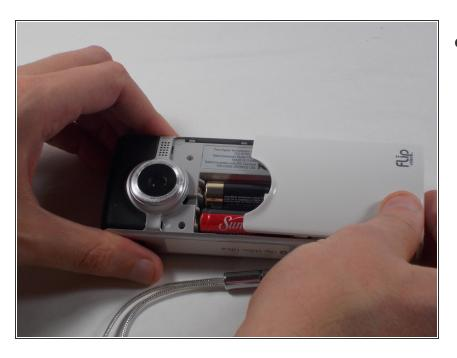
Remove the battery cover by sliding it down the camera.
