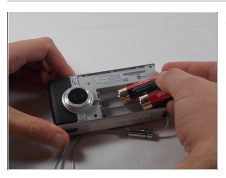
Remove the batteries.
