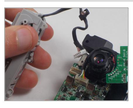
Fully remove the USB connector and replace it with the new USB connector. To reassemble your device, follow these instructions in reverse order.
