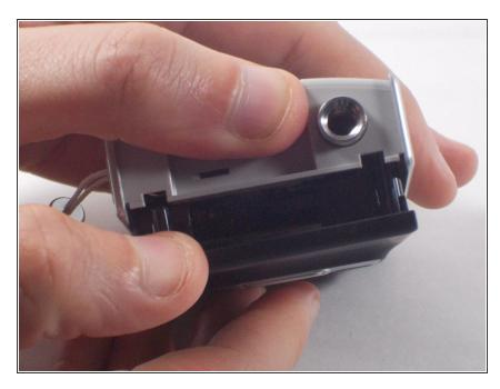
Remove the top casing from the bottom to reveal the inner circuit board.
