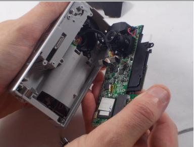
Gently separate the circuit board from the casing.
