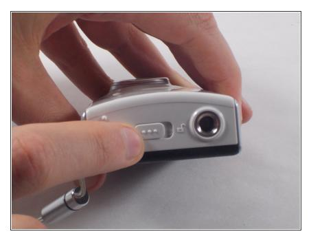
Unlock the battery cover by sliding the switch to the unlock position.
