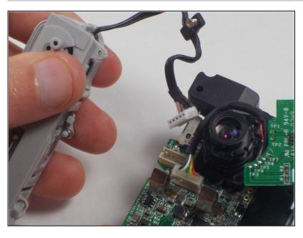
• Fully remove the USB connector and replace it with the new USB connector.
