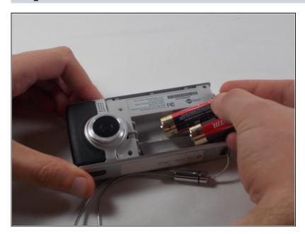
• Remove the batteries.
