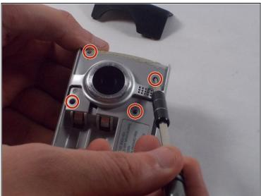
• Remove the six 1mm screws from front of the camera with the Phillips Head screwdriver.
