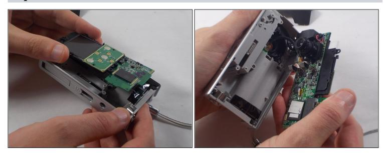
Gently separate the circuit board from the casing.
