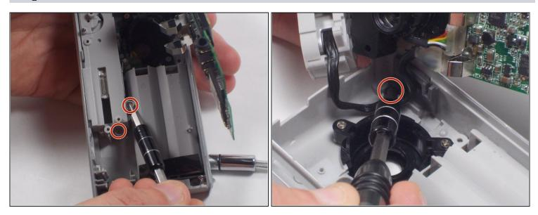
Remove the three 1mm screws from the USB connector and back casing with the Phillips Head screwdriver.
