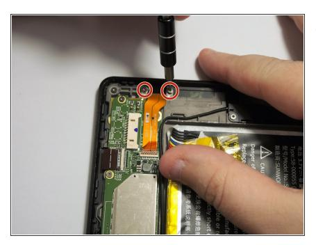
After locating the USB port at the top of the device, remove the (2) 3mm T4 Torx screws.
