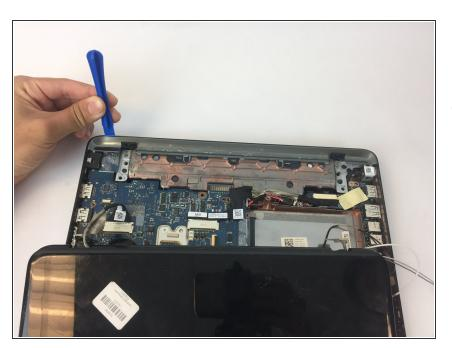
Lay the screen down and pry the left corner of the plastic casing that is located behind the screen.
