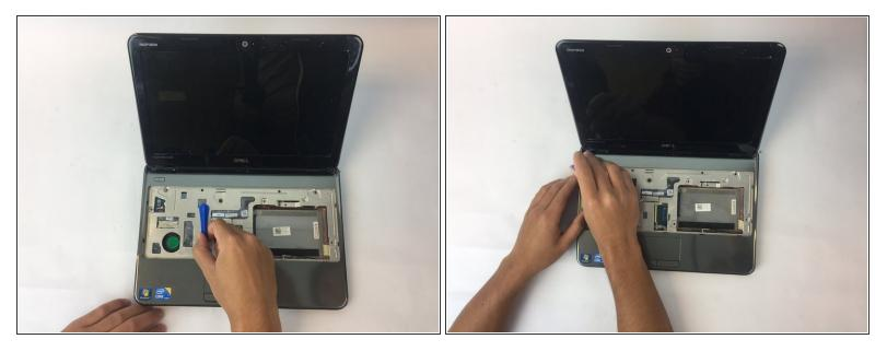
• Start by prying the outer casing of the laptop using the plastic opening tool. Start from the bottom and work your way around the edges.
