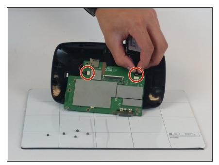
Disconnect battery wires from motherboard, so that you can remove the Lithium-Ion battery.
