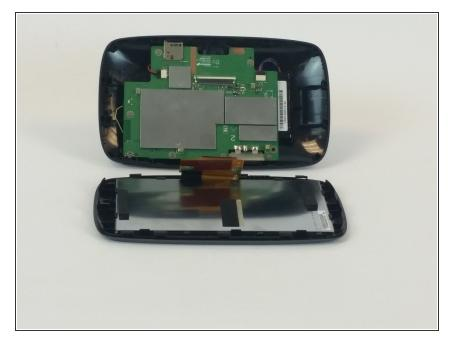
Your device should now look like this. Make sure to disconnect the screen from the motherboard by removing the flap connecting both, so you have ample room to work on the device.
