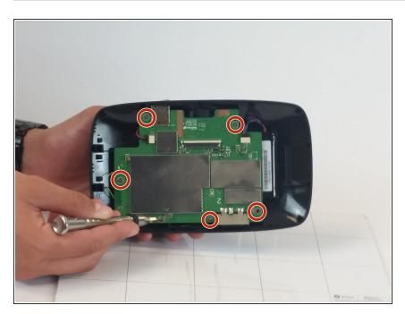
Remove all the screws that are marked in the image with a Philips #000 screwdriver and over a magnetic work mat.
