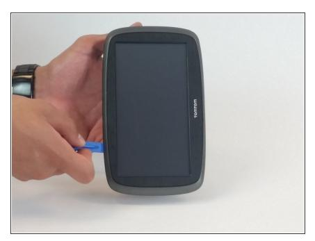
Use the iFixit opening tool to pry open the TomTom Go 60 S. Start from a corner and drag the tool around the device.
