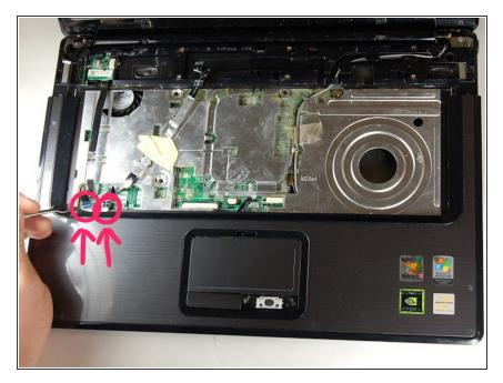
Separate the power connections.
