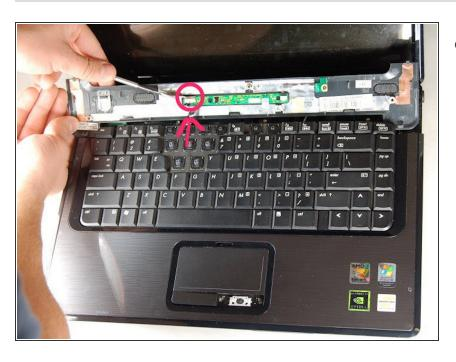
Separate the connection of the top piece from the board.
