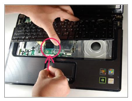
Remove the connection from the keyboard to its housing.
