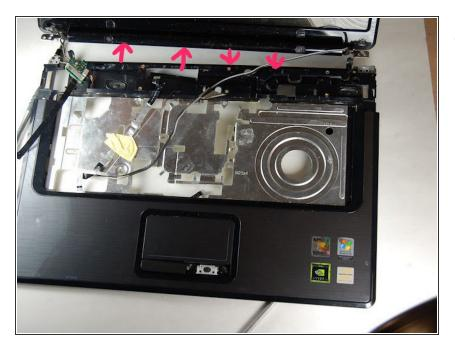
Make sure to grip the screen tightly and separate the top and bottom.
