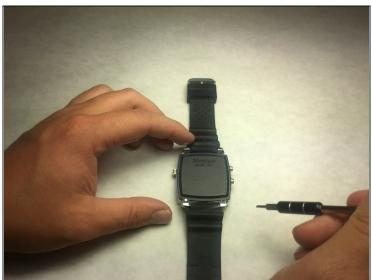
Unscrew the four 3.4 mm flat head screws
