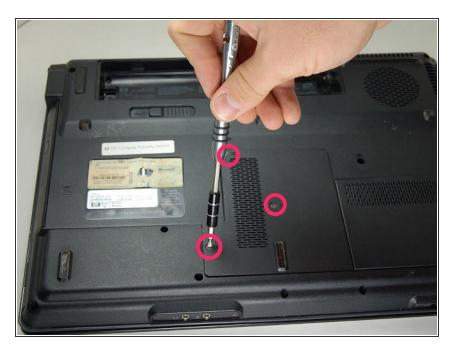
Grab a Type-Cross #1 screwdriver and unscrew the 3 screws and take off the cover of the wifi antenna card.
