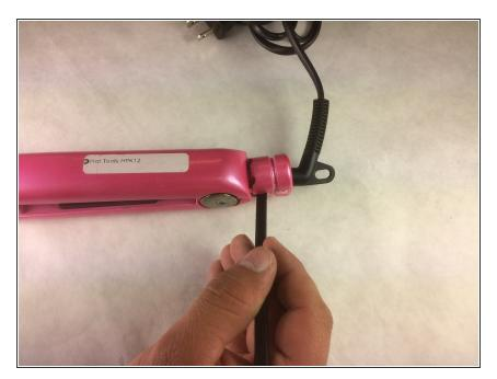
Separate the top and bottom pieces of the shell. It may require some force to break the seal.
