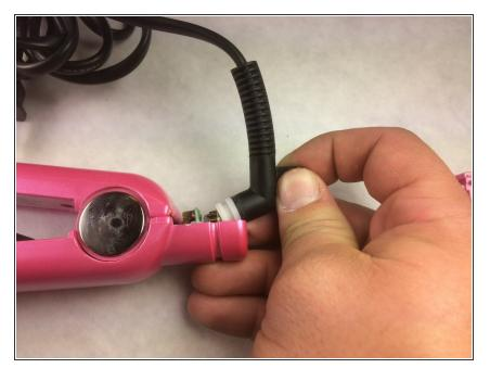
Remove the cord by pulling up and away from the bracket. You are now ready to replace the cord.
