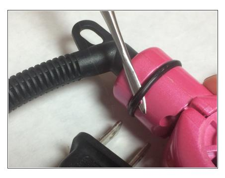
Slide the black O-ring out of its channel and pull it off the end of the flat iron.
