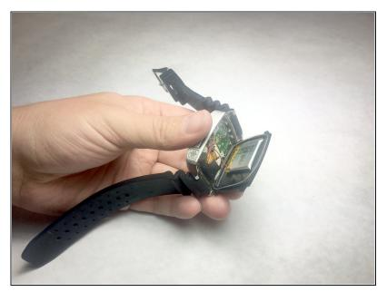
Carefully lift the back plate off the watch. You will notice a lithium battery and rubber gasket attached to the back plate.
