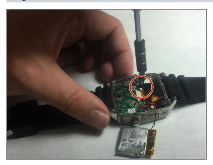
Use PH00 screwdriver to remove 5.2mm Phillips head screw
