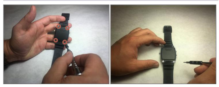
Unscrew the four 3.4 mm flat head screws
