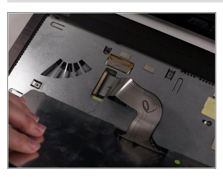
Gently pull the ribbon cable to the right and out of its port.
