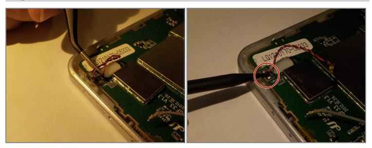
$\triangle$  Disconnect the positive and negative battery leads.
