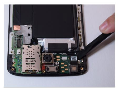
Use the spudger to delicately pry up the front-facing camera and remove it from the phone.
