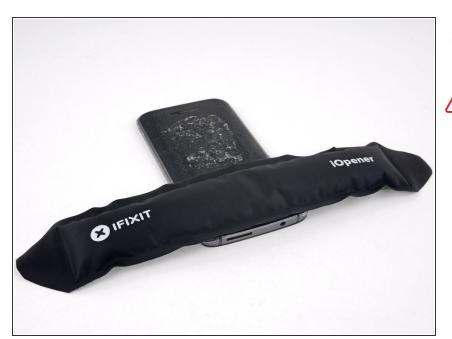
• <u>Heat an iOpener</u> and apply it to the top edge of the phone for a minute.
