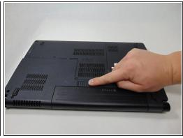
Slide the locking switch to the left to release the battery.
