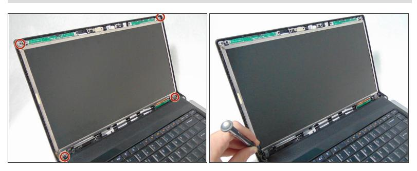
Remove the four 3 mm screws securing the LCD using the #1 Phillips screwdriver.
