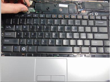
Remove the two 3mm screws with a #1 Phillips screwdriver, holding down the keyboard.
