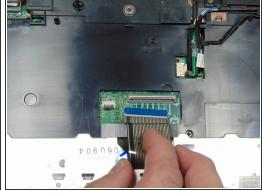
Flip up the black tab on the keyboard ZIF connector and unplug the cable.
