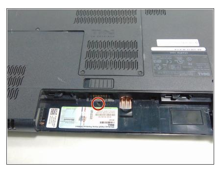
Remove the single 3mm screw underneath the battery with a #1 Phillips screw driver, which holds the media control cover.
