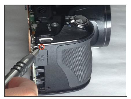
Remove the 3.0mm Phillips #000 screw located above the grey power flap on the side of the camera.
