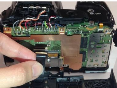
Gently pull the LCD ribbon connector up to allow the back casing to be completely removed.
