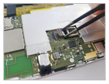
Use the precision tweezers to carefully pull out the connector and remove the camera.
