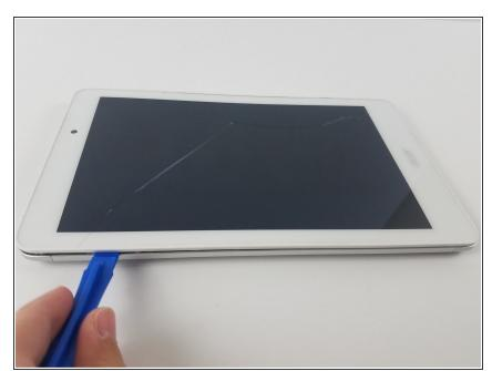
Wedge the plastic opening tool in between the display screen and back panel
