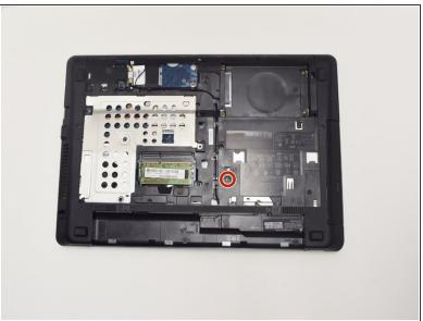
Remove one 6.0 mm Phillips PM2.5x6.0 screw that is securing the optical drive.
