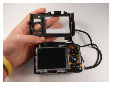
Remove back plate from the camera and locate the orange button plate to the right of the screen.
