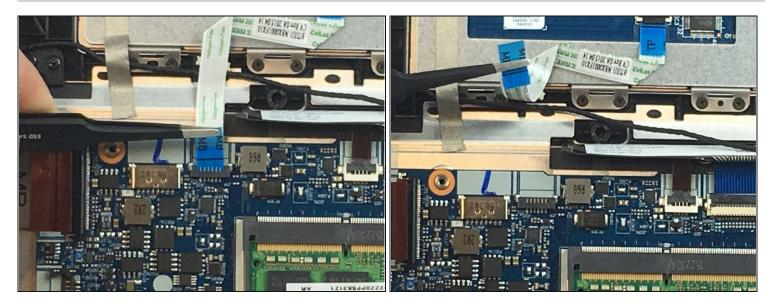
• Gently lift the clip holding down the blue ribbon connection the touch pad to the motherboard. Use tweezers to disconnect the ribbon.
