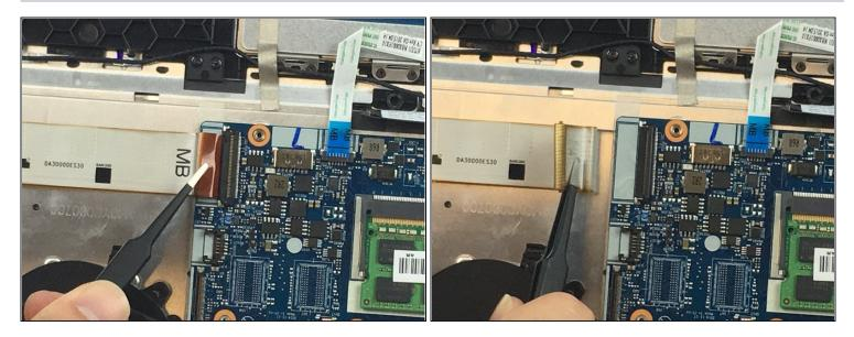
• Using tweezers, undo the plastic clip holding the ribbon in place and gently pull the ribbon to remove it.
