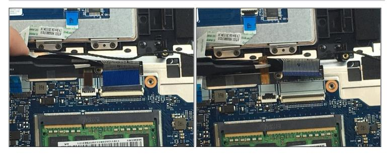
• Undo the clips holding the blue and brown ribbon to the motherboard. Use tweezers to gently remove both ribbons.
