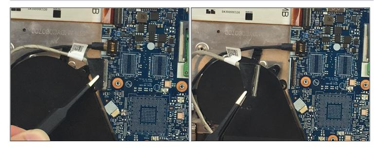
• Using tweezers, disconnect the second cable connecting the screen to the motherboard.
