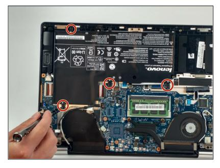
Remove the four 3mm PH#0 screws surrounding the battery.
