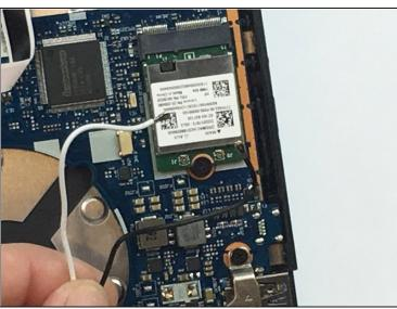
• Using the tweezers, disconnect the white and black cables connecting the motherboard to the screen.
