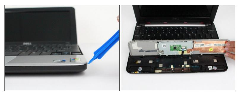
• Using a spudger, gently pry the palm rest off of the palm rest bracket.
