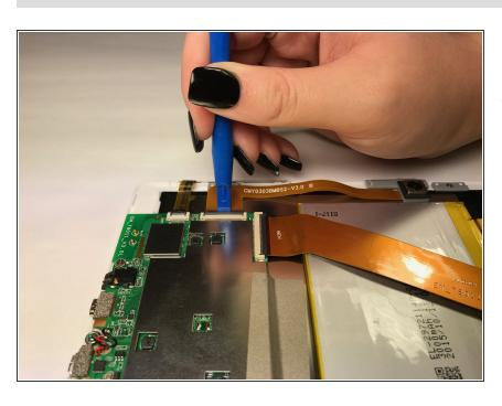
Using the plastic opening tool, lift up the black retaining flap that secures the camera ZIF (zero insertion force) ribbon connector to the motherboard.
