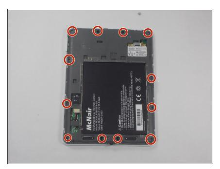
Using a Phillips #0 screwdriver, remove the 12 4mm screws on the outer area of the gray area exposed by removing the back panels.
