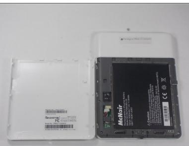
Remove the back panel by sliding it downwards and pushing in slightly.
