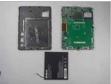
Now, lift up the gray piece, unplug the battery connector, and the battery can be removed from the case.
