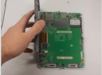
Carefully pry the back of the device from the front panel and motherboard. There are a series of clips holding them together that need to be separated.
